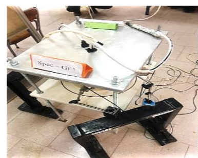
Figure ۶ - The location of the loading valves and the internal pressure measurement of the cylindrical shell
